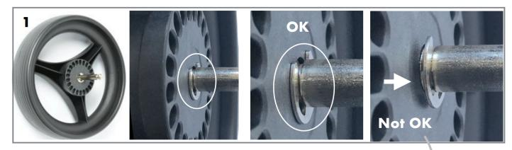
2 Add ring (see manual 127.1 - Disassemble wheel and axle)
